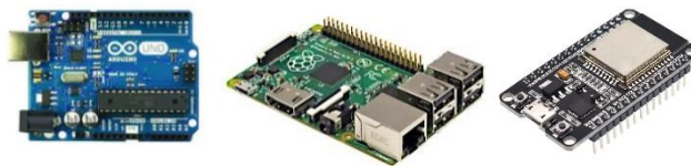
Fig. 3. Comparison of Arduino, Raspberry Pi, and esp32
