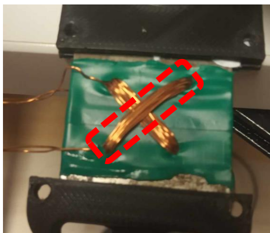
Fig. 9: The magnetoelastic sensor with the highlighted magnetizing winding.
