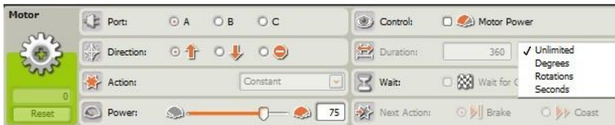
Fig.9 The range setting of Servo Motor properties
